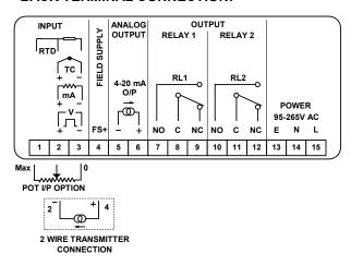
For valve position indicator input potentiometer should be minimum 1Kohm
